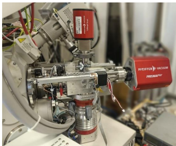
Fig. 1: Prototype of the HSID integrated into the ESEM chamber.
